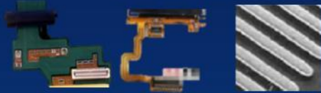
FPC with Fine line of 75/75µm
